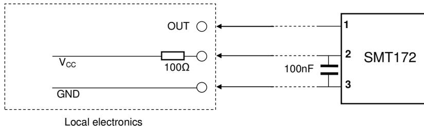
The capacitor will enhance the EMC performance and the resistor will also limit the maximum current in case of faults or wrong connections.
