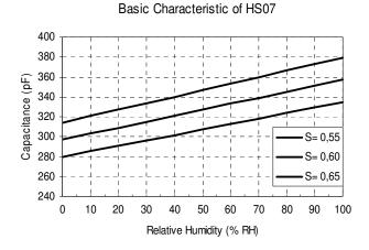
The measurement range is between 10% RH and 95% RH
